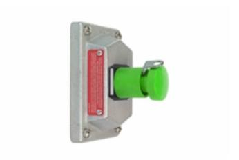
The EPS-PB10-GRN-SP0000 from Larson Electronics is an Explosion Proof Single Push Button Switch that is designed for use in hazardous work areas, such as chemical plants, oil refineries, and settings where combustible gases or dust may be present. This 10-amp device features the following explosion proof ratings: Class I Divisions 1 and 2; and Class II Divisions 1 and 2. Device box sold separately.
