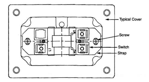
**CAUTION:** Use 12 AWG copper conductors only. Insert the bare wire conductor(s) under the terminal clamp and securely tighten the screw(s). Note: Do not exceed 35 in-lbs. of torque.
