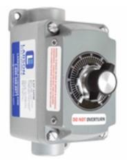
EXP-DRW Explosion Proof 0-10V Rotary Dimmer Switch Switch Type: 0-10V Dimmable Rotary Switch Max Lamps per Switch: 25 Grounding: Single Internal Housing Ground Screw Dimensions: 5.88" L x 3" W x 2.25" D Configuration: Front Mounted Rotary Switch Hub Quantity: (2) Feed Through or (1) Dead End
