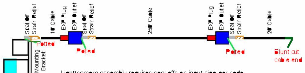
Light/camera assembly requires seal offs on input side per code Additional potting at cable entrace of light/camera assembly with an epoxy potting compound.
