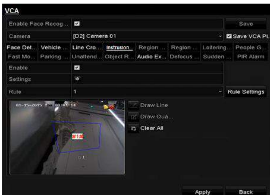
Figure 9. 4 Draw Area for Intrusion Detection
