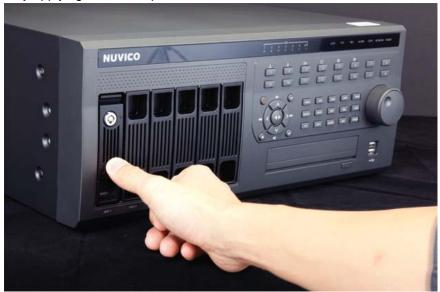
5. Finally, use the supplied tray key to lock the HDD tray into the chasis to prevent unauthorized removal.
