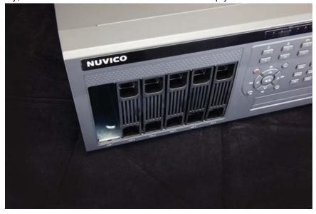
3. With the latch pointing upwards, slide the tray into the slot.
