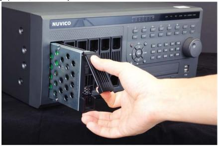
4. Lock the tray in the slot by applying downward pressure to the latch.
