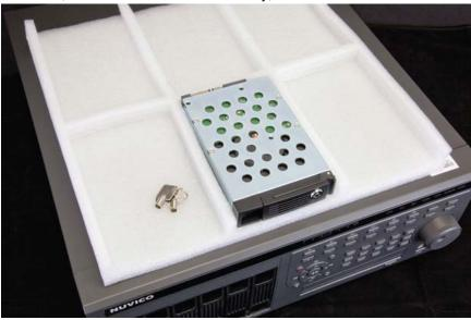
2. The removable HDD tray, shown below needs to be inserted into the empty slot of the DVR.
