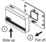
Pass the wires through and fix the mounting plate to the wall.
