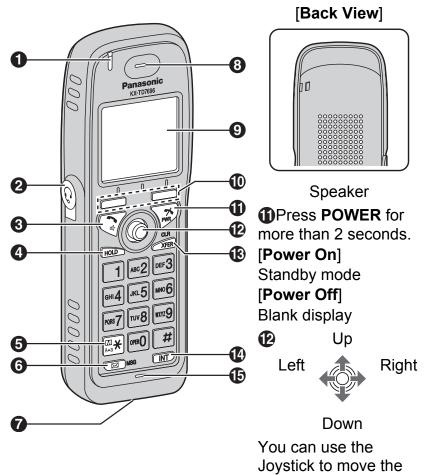
Joystick to move the cursor in the desired direction. Press the center button to confirm a selection.
