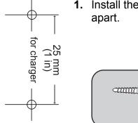
1. Install the two included screws in the wall, spacing them 25 mm (1 in) apart.
