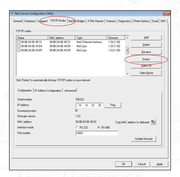
made in the DHCP server, to ensure that the same IP address is issued each time, should the unit be reset. Consult your network administrator on detail of how to reserve IP addresses. The unit's MAC address can be read from inside the plastic enclosure, and will be required by the Network administrator to enter the reservation.
