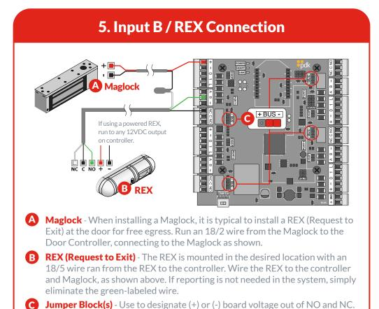
If the jumper is off, the relay is a standard dry contact needing input into
