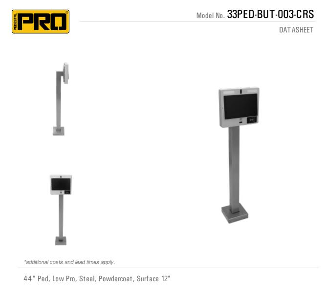
44" tall steel pedestal with a low profile neck (3") reach. Powder-coated to color match the touch panel. Made from heavy duty 3x3 steel tube, with 6x6 faceplate and 8x8 base with cover plate.
