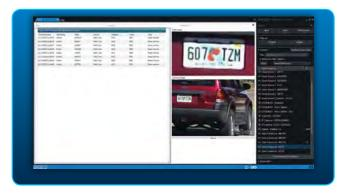
This full-frame plug-in allows real-time monitoring of license plates read by all cameras on the ARES system. The Plate Viewer Plugin goes beyond capturing plate number and state, province or country, to display the critical data to make actionable decisions.
