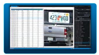
One of the key features of the ARES system is the ability to define rules that are run against LPR data. As license plate reads occur, they are checked against the active rules, and an alert is generated if they meet the specified criteria, allowing for real-time monitoring alerts.
