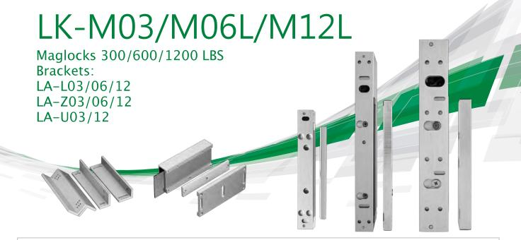
Rosslare's LK-M03/M06L/M12L high quality magnetic locks are ideal for secure applications where access is restricted, such as office buildings, hospitals, and airports. They have a holding force of 300/600/1200 pounds, respectively, and are easy to install. The attractively designed Maglocks are surface mounted, operate on dual voltage, 12 VDC or 24 VDC, and have low current consumption. These Maglocks are compatible with EN and UL standards.
