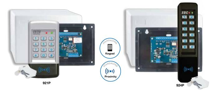
The SDC 921P and the 924P EntryCheck™ are indoor/outdoor stand-alone digital keypads with Prox Reader and Controller (2-piece configuration), designed to control access of a single entry point with up to 500 users. Each user is assigned a proximity card and/or a personal identification number (PIN). Presentation of a proximity card or keypad entry of a code activates one or both of the output relays which releases an electric door lock.
