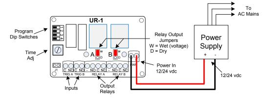
WARNING!: The UR board Output Relays must be protected against inductive kickback generated when power is removed from an inductive load (e.g., electric strikes). Refer to the lock manufacturer's installation manual or contact the manufacturer for kickback protection recommendations.
