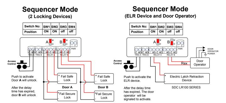
WARNING!: The UR board Output Relays must be protected against inductive kickback generated when power is removed from an inductive load (e.g., electric strikes). Refer to the lock manufacturer's installation manual or contact the manufacturer for kickback protection recommendations.
