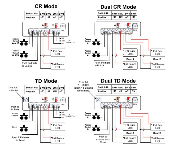
WARNING!: The UR board Output Relays must be protected against inductive kickback generated when power is removed from an inductive load (e.g., electric strikes). Refer to the lock manufacturer's installation manual or contact the manufacturer for kickback protection recommendations.
