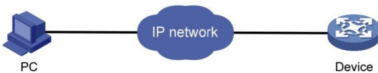
Figure 1-1 Web Management Operating Environment
