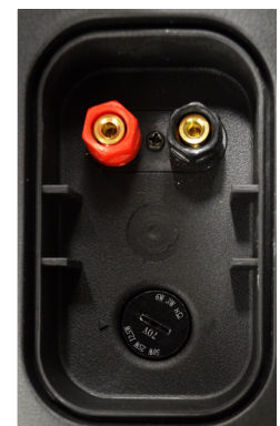
close-up image of transformer and wire terminals
