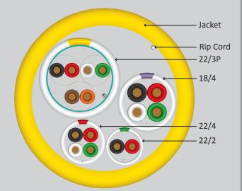
ACCESS CONTROL CABLE PLENUM 22 AWG/3P Shielded + 18 AWG/4C + 22 AWG/4C + 22 AWG/2C
