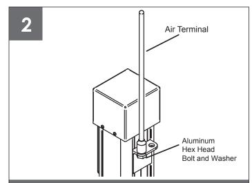
Place the air terminal in one of the holes on the aluminum angle bracket. Attach the washer and hex head bolt and tighten securely.
