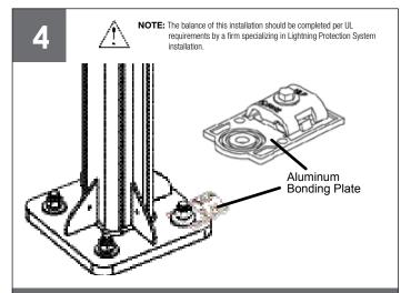
Scrape away any paint from the area underneath the fourth bolt. Place the aluminum bonding plate over the fourth bolt and secure using washers and the fourth bolt.
