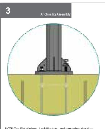
NOTE: The Flat Washers, Lock Washers, and remaining Hex Nuts will be used to fasten the pole to the Anchor Jig.
