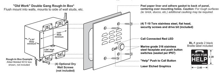
\* Caution: Excessive wire length and/or using a rough-in box with inadequate depth can apply force to the circuit board causing physical damage.
