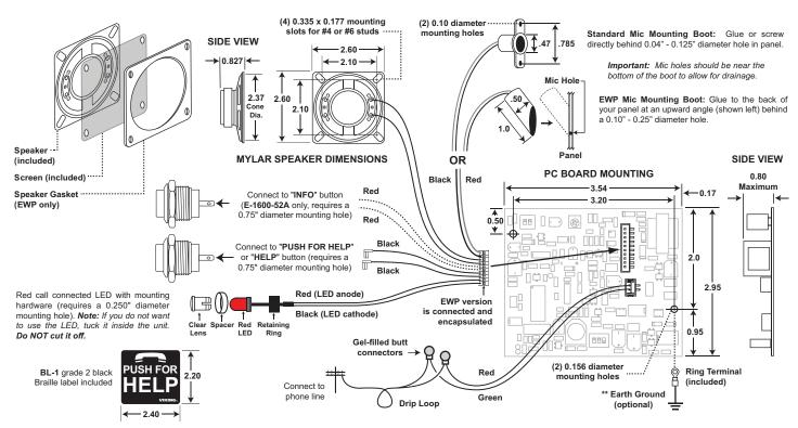
\* Important: If installing the EWP version outdoors, apply a non-corrosive silicone to back side of LED and push button switches after making all connections and testing. Completely encapsulate exposed switch connections (terminals/stripped wires) and bare wire connections.
