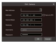
Select the device you want to add and then click the "Add" button. The NVR will automatically refresh the cameras and return to the "Edit Camera" interface. "Online" status means connecting the device successfully and you will see the live image. You may select the added device and click button to modify channel, IP address, etc.
