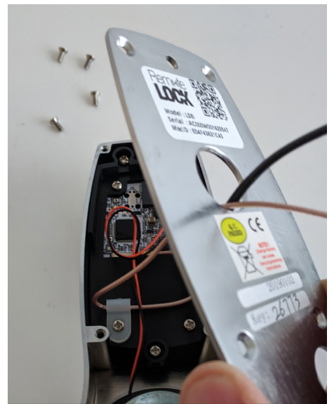
11. Re-thread both cables through the top hole and fix the backplate back using the 4 screws.
