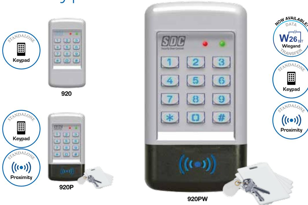
The SDC EntryCheck™ 920 Series indoor/outdoor digital keypads are designed to control access of a single entry point with up to 500 users. Each user is assigned a personal identification number (PIN). Keypad entry of a valid one to six digit code activates one or both of the output relays which releases an electric door lock. Featuring heavy cast vandal resistant housing and cast metal blue backlit keys.
