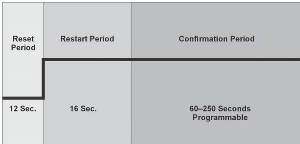
Figure 10.99 Smoke Verification Cycle
