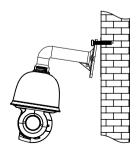
(5) Connect the cables and then hang the bracket on the wall .
