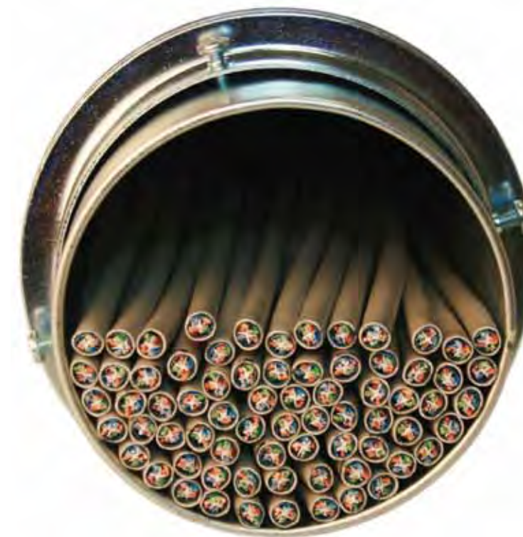
10Gain XP CAT 6A cable allows 71 cables in 4" conduit at a 40% fill rate.
