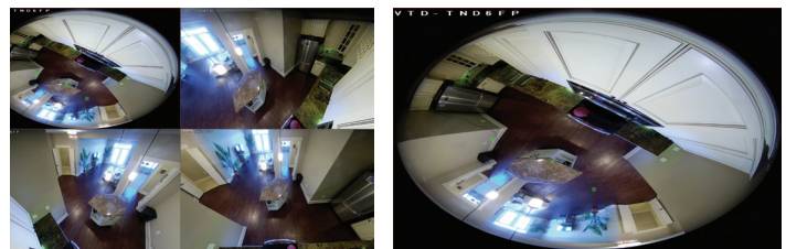
Fish Eye De-Warping: Multiple Views include 360° Overview, Double 180° Panorama View, Quad View, Overview + 3 Views, and Single View
