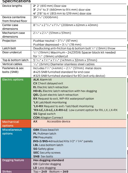
\*For 33/3549A devices, LX switch monitors trim input or electric dogging of EL/QEL devices. LX switch does not monitor latchbolt condition.
