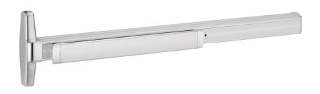
3349A and 3549A for hollow metal single and double doors, UL listed for panic exit hardware. Devices are ANSI A156.3 – 2008 (LBL option 2014) Grade 1. The 3549A has a smooth mechanism case and the 3349A has grooved case. The concealed vertical cable device is non-handed except when the SS (signal switch) option is used. See opposite page for available outside trim and device
